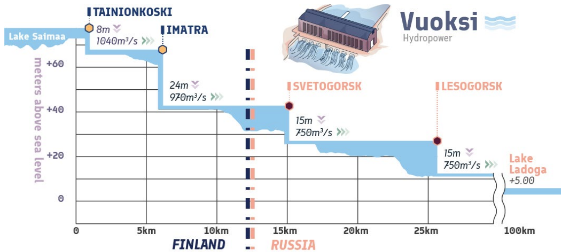
Figure 2 Profile and hydropower plants of the Vuoksi
